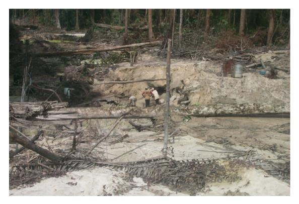
Photo 6 – Unsafe operating pit conditions, at Baramalli.
