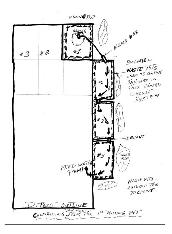
Sketch 1: A System For Retaining Tailings From the First Mining Pit, With Ore-body Demarcated and Backhoe Available
