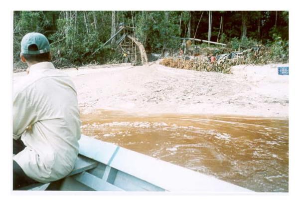
Photo 2 – Tailings Discharged Directly into Kurupung River
