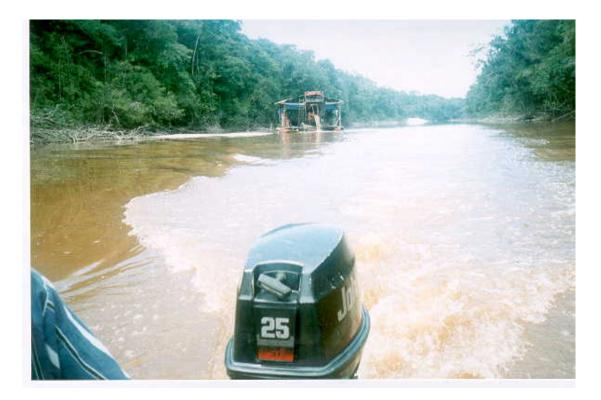
Photo 28 – Improper Positioning of River Dredge, with Tailings Discharge Angled Towards River Channel, Kurupung River.
