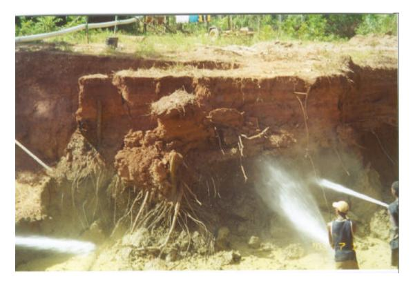
**Photo 24** - A Typical Land Dredging Operation at Arakaka, where both Overburden and Pay Material are Removed by Jetting and Routed Through Sluice Box.
