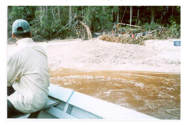
**Photo 10** – Tailings Discharged Directly into the Kurupung River by Roger Baxter's Operations.
