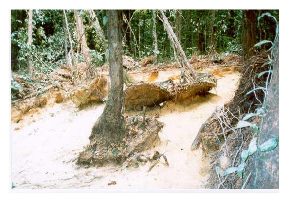
Photo 18 – Undermined Trees Left Standing in a Mined-Out Pit, at Chance Creek.
