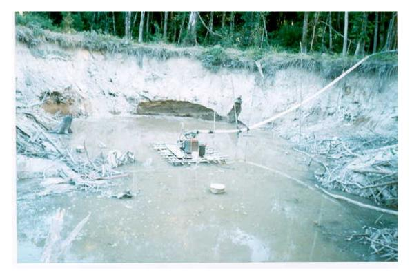
Photo 4 – Mine Pit of Roger Baxter's Operations on the Kurupung River Bank. Water Percolating From The River Aid in The Collapsing of Walls of The Thick Overburden Cover.
