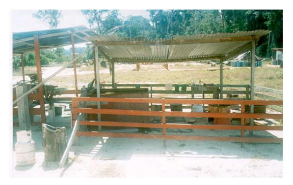
Photo 19 – Retorting Shed Consisting of Mercury Retort, Jig Box and Shaking Table for Proper Processing of Gold Amalgam and Black Sands. (CMC's Operations at Olive Creek).
