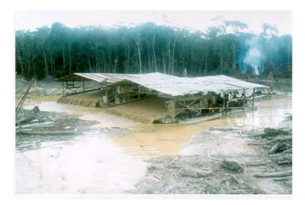
Photo 17 – Totally Enclosed Operation of Two Missile Dredges, with Wide Sluice Discharges, Operating in Tandem, at Correia Mining Company, Olive Creek.
