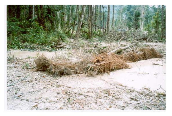
Photo 8 – A Rapid Filtration Dam, Constructed From Fibrous Roots and supported by Tree Trunks, as Part of a Closed-Circuit Recycled Water System. Raimundo DaSilva's Operations at Upper Takuba Creek.
