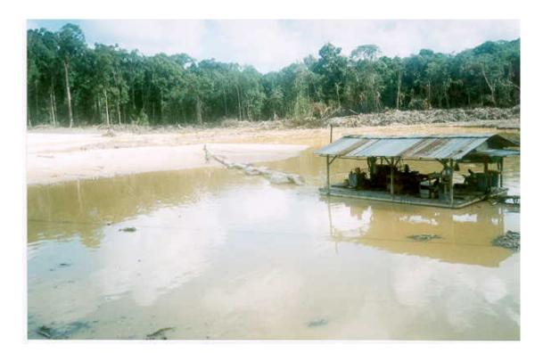
Photo 13 – Ordinary River Dredge, with Extended Floating Discharge Line, Converted to a "Bailer" for Repositioning Tailings, From Missile Dredges, Away From the Mine Pit. CMC's Operations at Olive Creek.
