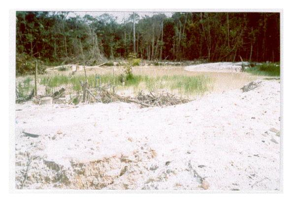
**Photo 9** – Tailings to be Routed Through a Patch of Grass to Aid in Filtration and Settlement of Tailings Solids. DeAssis Lopes' Operations at Barlow.
