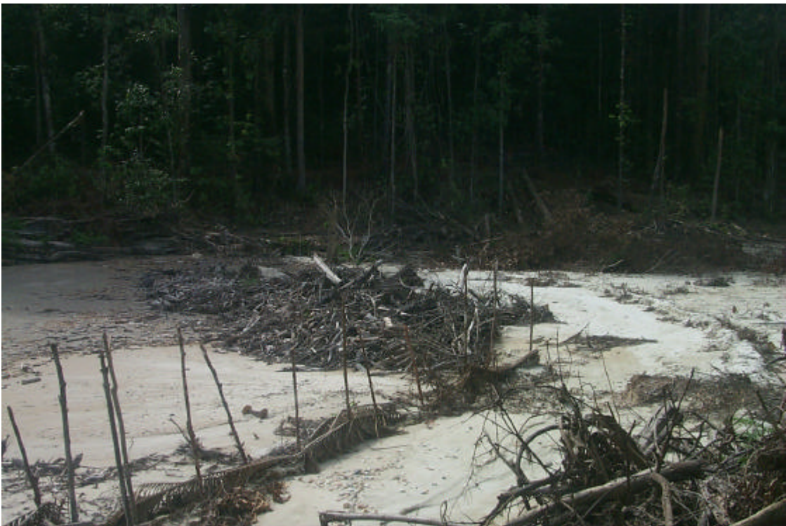
Photo 4 – Crude system of indigenous material used to confine tailings solids at Filho’s operation, Baramalli.
