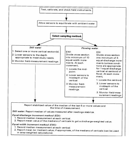
Figure 6.2: In Situ Field Measurement Procedures for Surface Water
