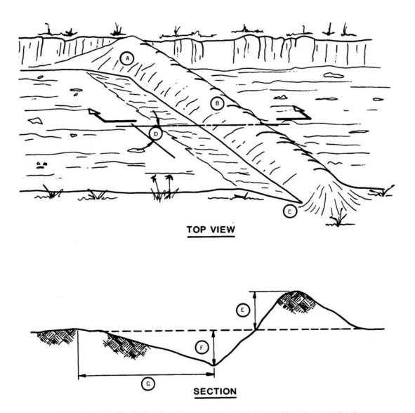
WATERBAR (CR05SDITCH). Construction for unpaved forest roads with limited or restricted traffic. Specifications are average and may be adjusted to gradient and other conditions. <u>A</u>, bank tie-in point cut 6 to 12 in. into roadbed; <u>B</u>, cross drain berm height 12 to 24 in. above roadbed; <u>C</u>, drain outlet cut 8 to 16 in. into roadbed; <u>D</u>, angle drain 30 to 40 degrees downward with road centerline; <u>E</u>, height up to 24 in; <u>F</u>, depth to 18 in; <u>G</u>, 36-48 in.
