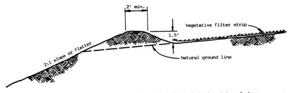
NOTES: 1) Dike constructed by dozer moving soil upslope and dumping at top of slope. 2) Outlet to stabilized vegetated soil.
