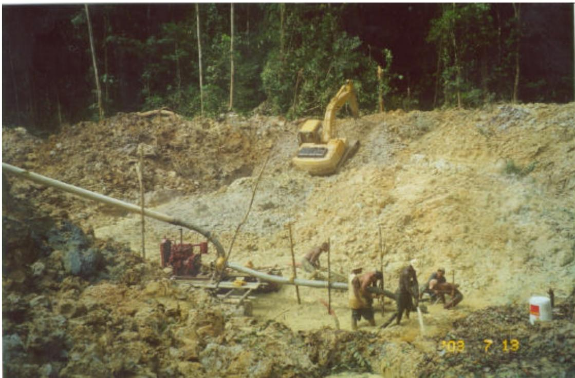
**Photo 4** - The Impact of Mechanization: The use of Cat. Backhoe (M. Seenarine's Operation at 14 Miles) to separate Overburden from Pay Material, Enabling Only Pay Material to be Removed by Jetting then Routing to Sluice Box.
