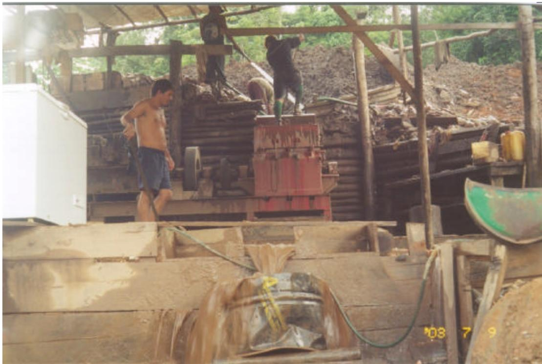
**Photo 8** - The Impact of Mechanization: The use of Small (Jaw) Crushers (J. Jairam's Operation at Purple Heart) Enables Processing of Previously Unmanageable Hard Rock Deposits.
