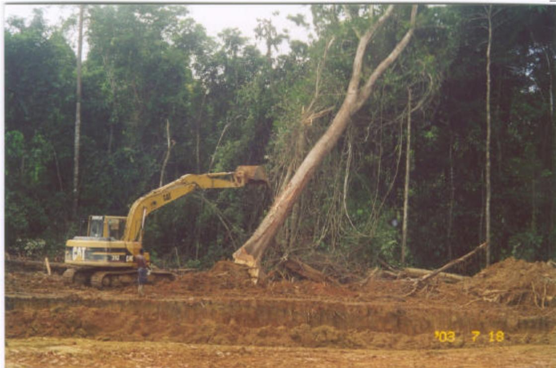
**Photo 6** - The Impact of Mechanization: The use of Cat. Backhoe (C. Adams' Operation at Five Star) Allows Good Pit Definition and (in Combination with a Power Saw) Effective and Safe Debushing.
