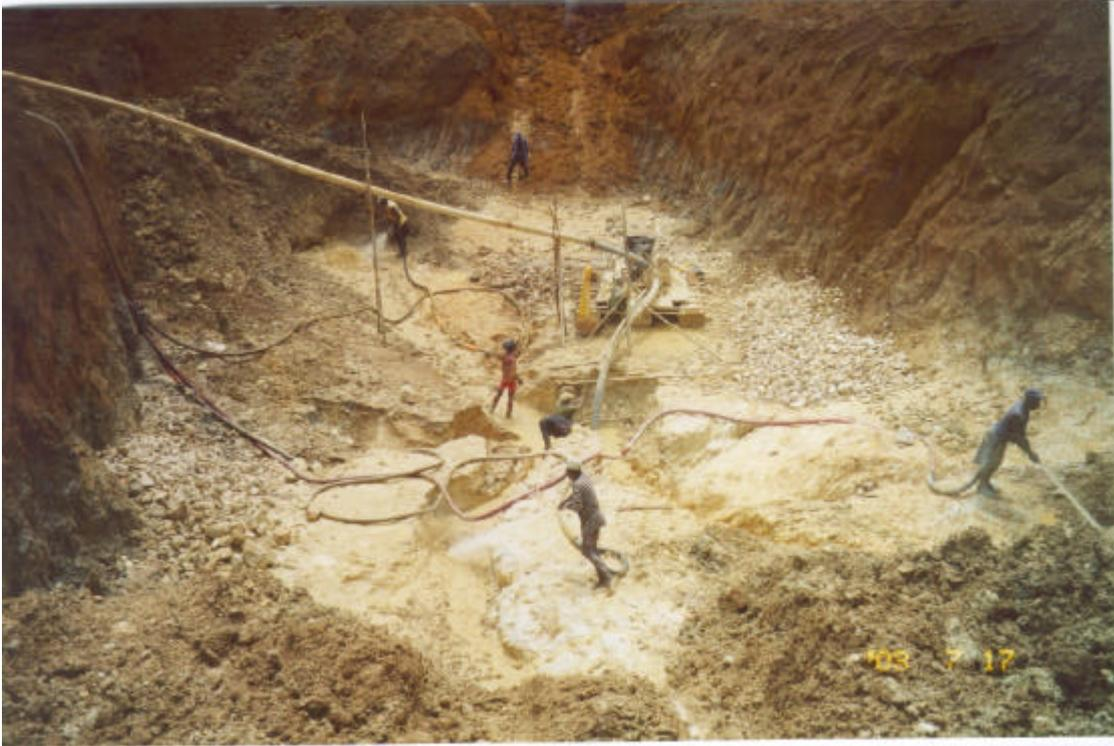
**Photo 5** - The Impact of Mechanization: The use of Cat. Backhoe (C. Adams' Operation at Five Star) Resulting in Clean and Stable Pit Walls, with Jetting of Pay Material Only.
