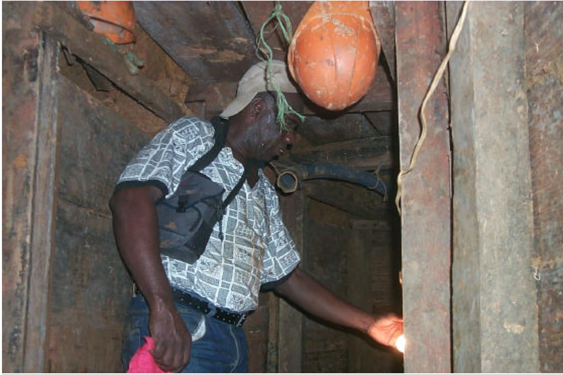
**Photo 9** - A Fully Supported, Artificially ventilated and lighted Vertical Timber Shaft and Adit System in Hard Rock Operation. (Edenilson Santos Pereira's Operations at Eyelash).
