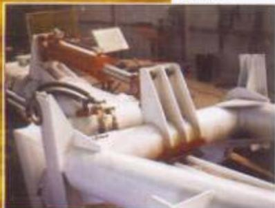
Multi-articulated ladder head and operating cylinder during construction
