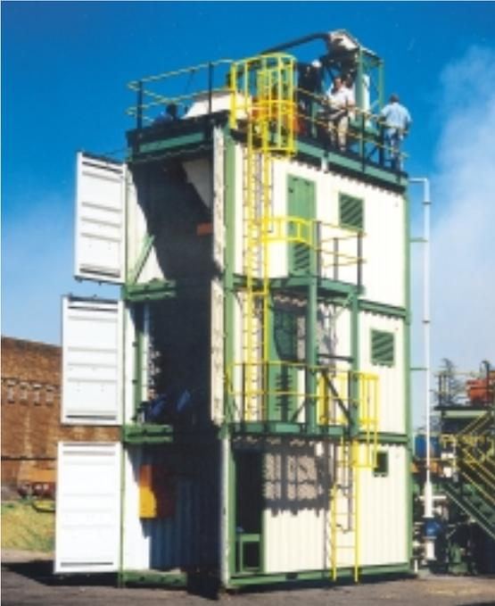
*A containerised x-ray recovery unit. Easy access for maintenance of equipment is provided through the double doors at the ends of the containers.*
