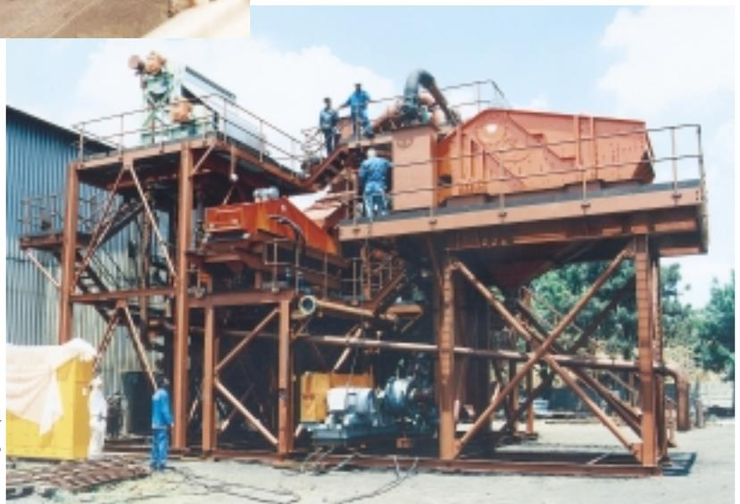
*The 150 t/h BATEMAN DMS plant featuring two cyclones fully erected at the fabricator's site before transport to MIBA, Mbujimayi, DRC.*
