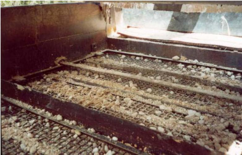
e) Jig top mesh replaced and ready for operation
