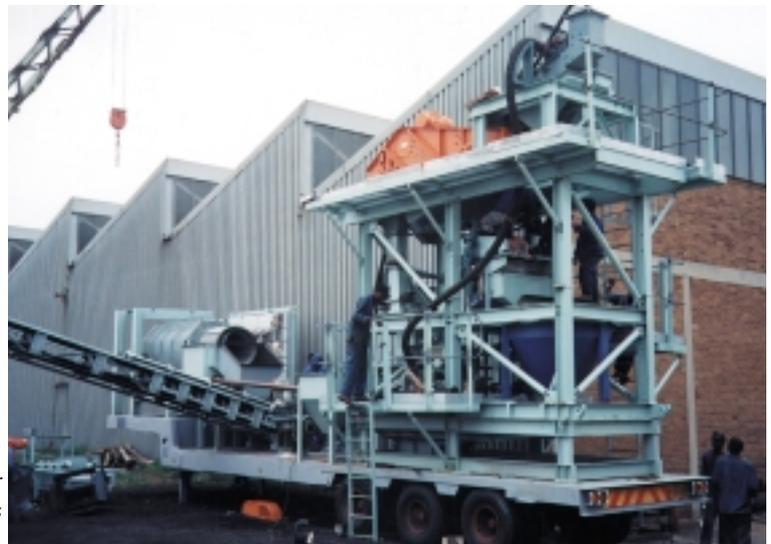
*Factory testing the trailer-mounted modular diamond sampling plant. This plant was supplied to Alexkor, Alexander Bay.*
