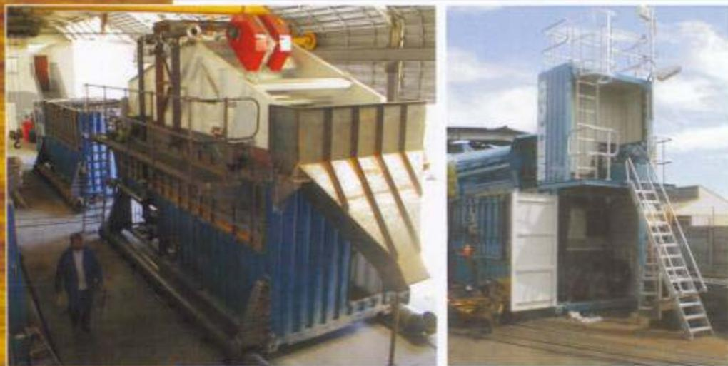
*MB 200 In-Field screening plant under construction in ADP Projects Cape Town factory.*
