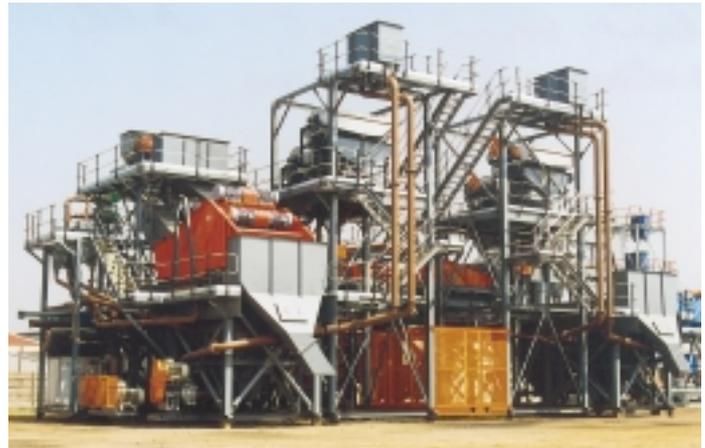
*Trans Hex Mining's twin 150 t/h DMS modules, trial erected at the factory.*
