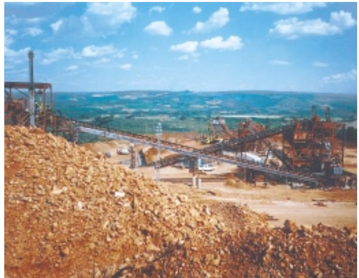
*MIBA's 400 t/h kimberlite process plant at Mbujimayi, DRC.*
