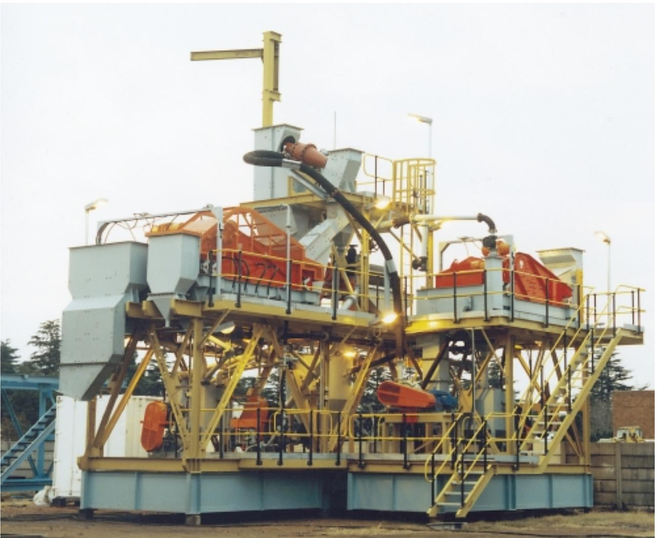
*A 50 t/h DMS module in the fabricator's yard, ready for delivery.*
