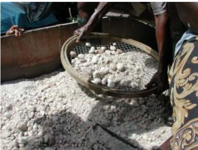
c) Removing the jig bed
