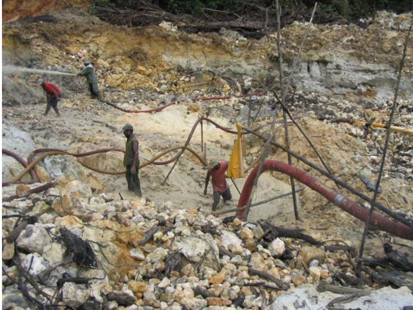
Photo 2-1 Land dredge mining
