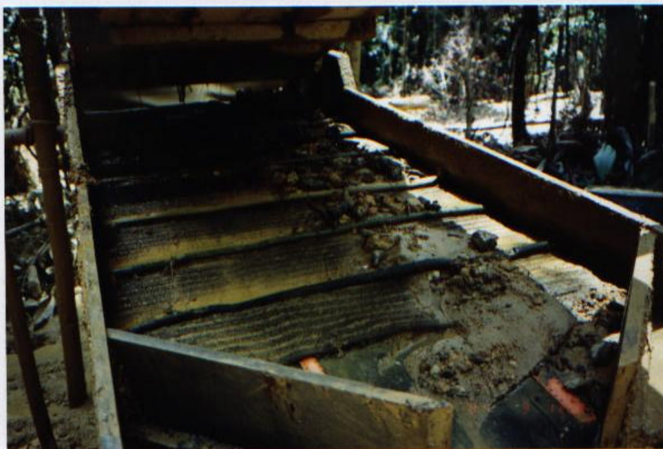
Photo 8 – Cross Ribs on Katchia's Sluiceway
