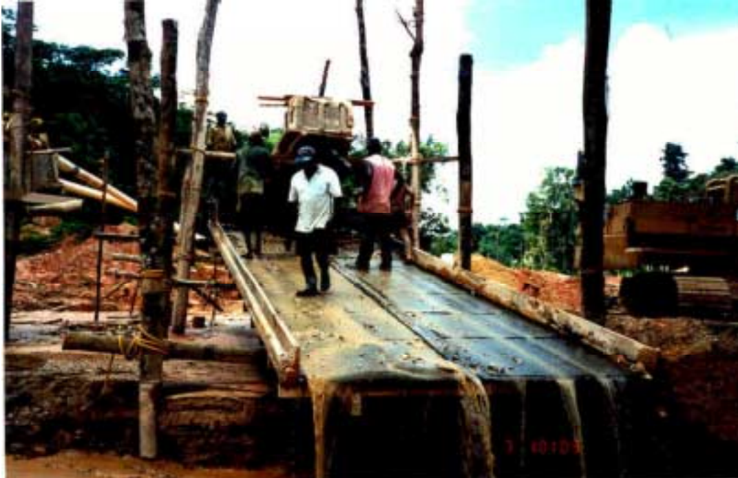
Picture 4: Mr. Insanalli's lower sluiceway narrowed to 6 feet in width and fitted with coarse expanded metal riffles over unbacked Nomad matting, lowest section is carpet.
