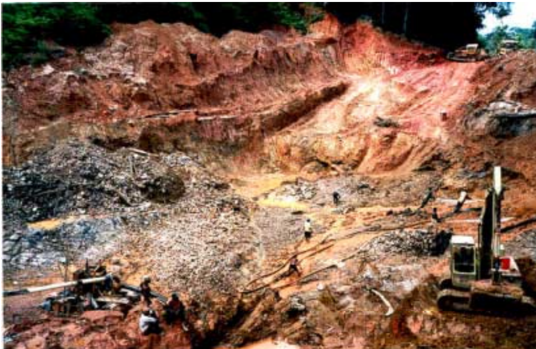
Picture 2: Mr. Insanalli's Open Pit with quartz vein exposed on lower left, jetting on right assisted by excavator and bulldozer (top right), and gravel sump on lower center.
