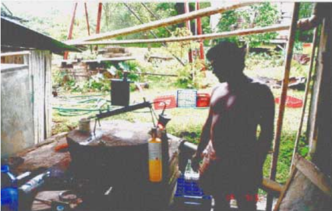
Picture 18: Demonstration of mercury resort that is being heated with a small plumber's propane torch at Bryan Phillips' operation.
