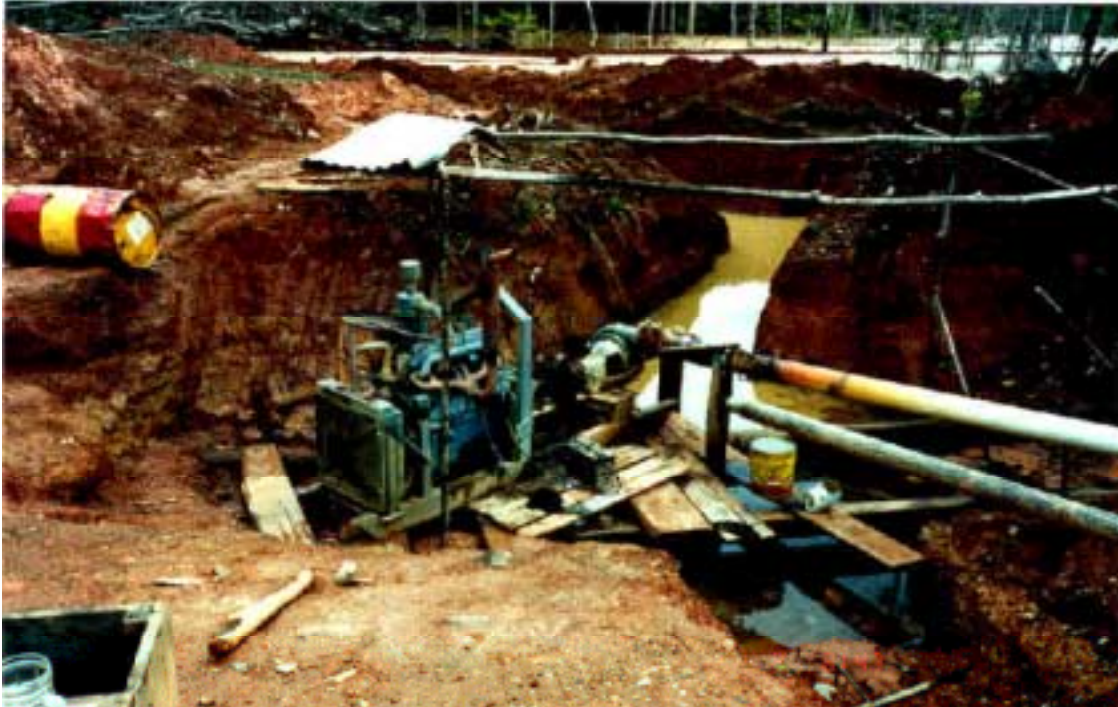
Picture 8: Mr. Insanalli's top section narrowed to 4 ft in width and refitted with one-inch angle iron riffles over unbacked Nomad matting, yellow ribbons indicated radiotracers.
