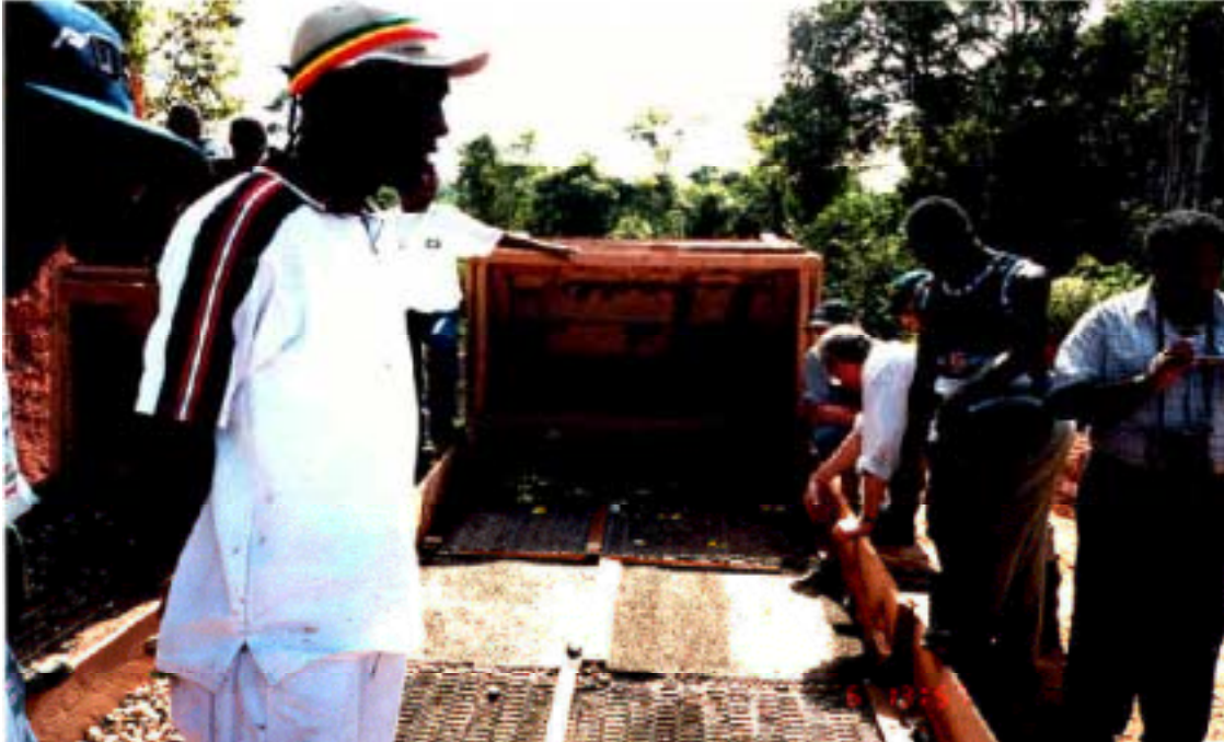
Picture 14: Upgrading sluicebox concentrates and testing refitted sluicebox with a small sluicebox (Long Tom) at John Phillips' mine.
