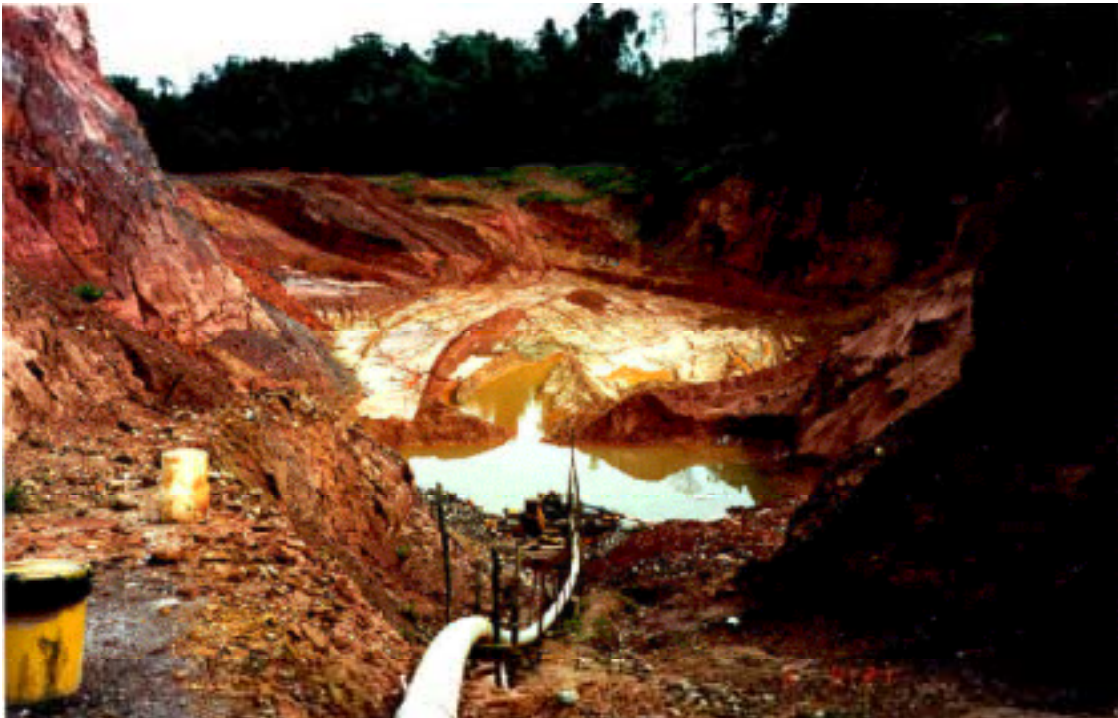
Picture 2: Mr. Insanalli's Open Pit with quartz vein exposed on lower left, jetting on right assisted by excavator and bulldozer (top right), and gravel sump on lower center.
