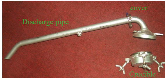
Picture showing main components of retort
