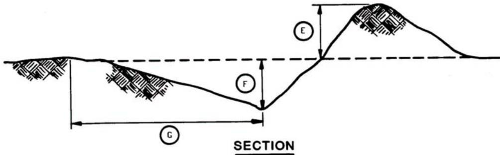
WATERBAR (CROSSDITCH). Construction for unpaved forest roads with limited or restricted traffic. Specifications are average and may be adjusted to gradient and other conditions. A, bank tie-in point cut 6 to 12 in. into roadbed; B, cross drain berm height 12 to 24 in. above roadbed; C, drain outlet cut 8 to 16 in. into roadbed; D, angle drain 30 to 40 degrees downward with road centerline; E, height up to 24 in; F, depth to 18 in; G, 36-48 in.
