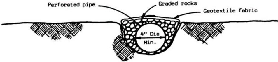
NOTE: Diameter of pipe to be based on the amount of water to be drained.
