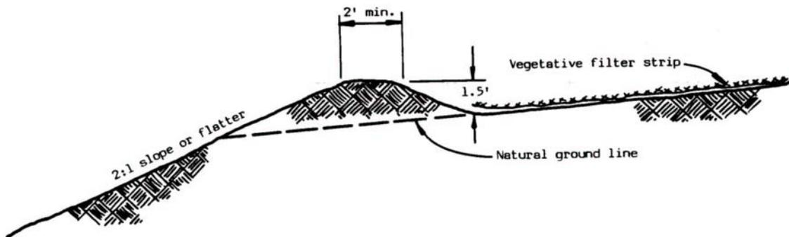
NOTES: 1) Dike constructed by dozer moving soil upslope and dumping at top of slope.
