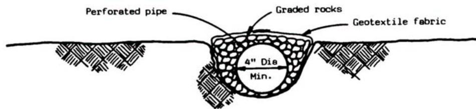
NOTE: Diameter of pipe to be based on the amount of water to be drained.
