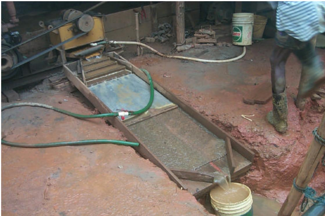
**Photo 26** – Mercury Plate For Gold Amalgamation in Crusher Processing System at Eyelash. Note brown spots indicating loss of mercury.
