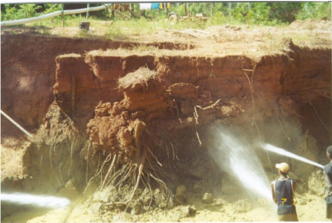
**Photo 24** - A Typical Land Dredging Operation at Arakaka, where both Overburden and Pay Material are Removed by Jetting and Routed Through Sluice Box.
