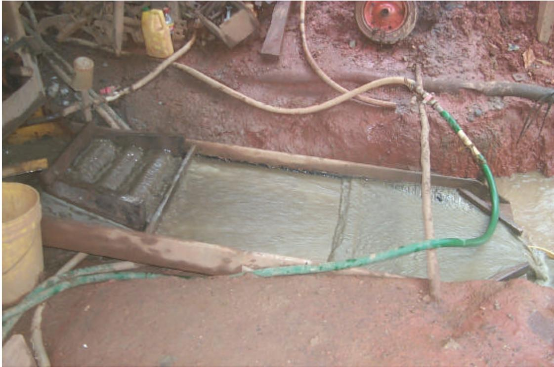
**Photo 27** – Mercury Plate in Operation at Eyelash.
