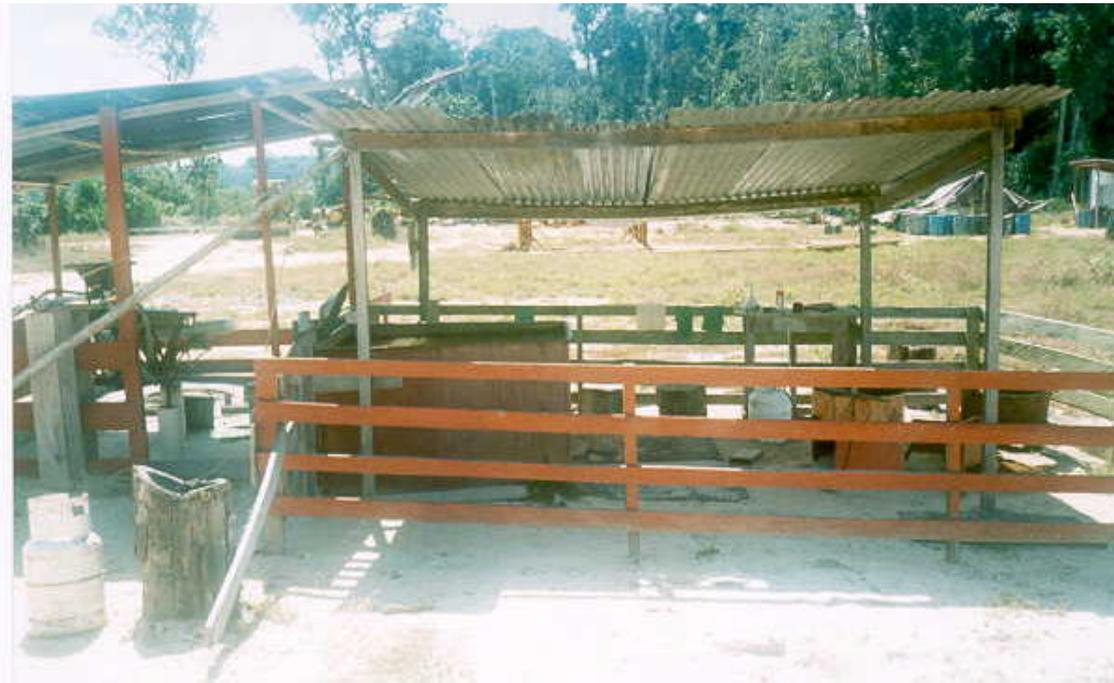
**Photo 10** – Retorting Shed Consisting of Mercury Retort, Jig Box and Shaking Table for Proper Processing of Gold Amalgam and Black Sands at Olive Creek.
