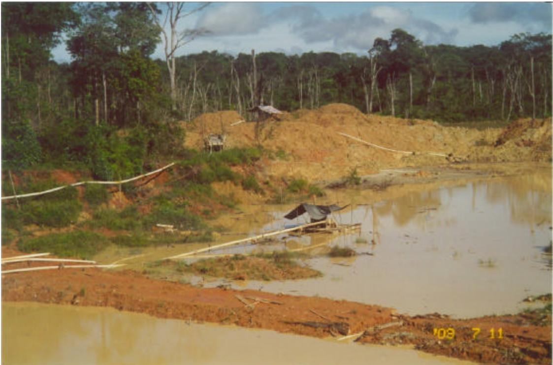
**Photo 22** – Old Mined-out Pits Used to Establish Closed Circuit Recycle Water System at Arakaka
