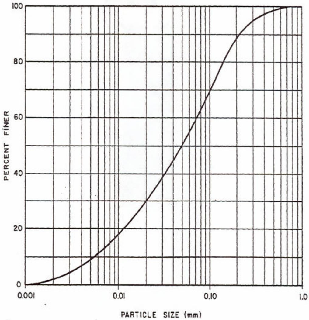
**Figure 4:4 Settleable Solids Size Distribution**
