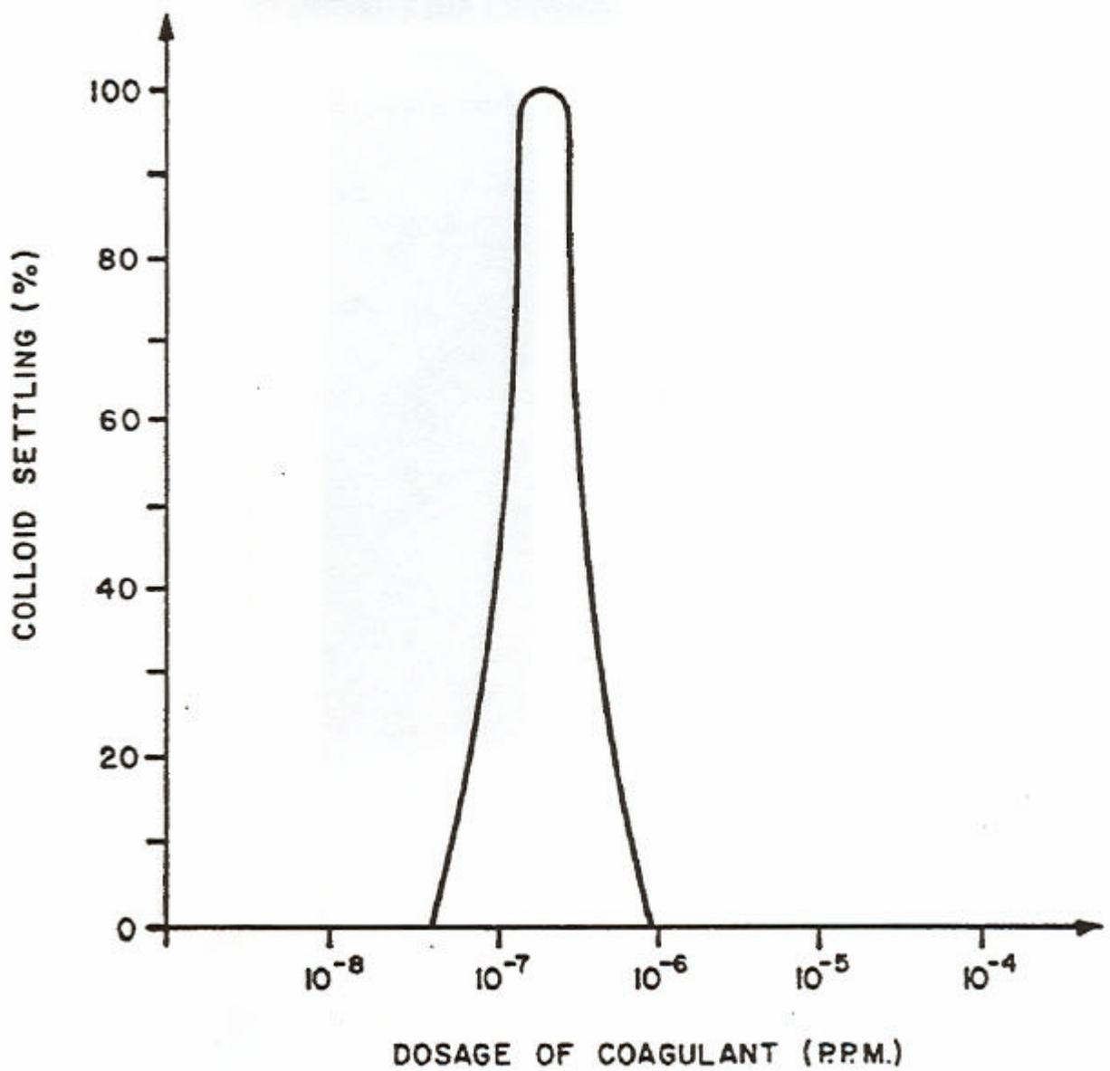
**Figure 5:1 Effective Concentration Range of Coagulants and Flocculants**
