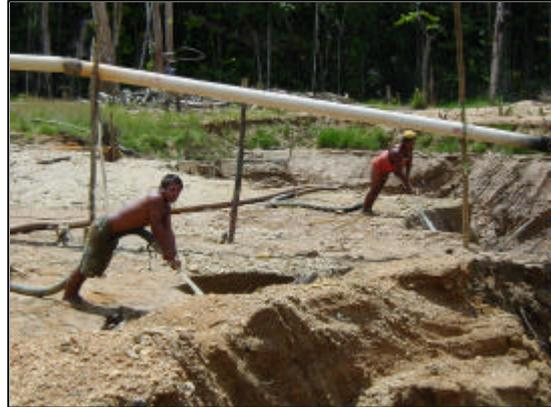
Picture 6.2: Topsoil hydraulicking
