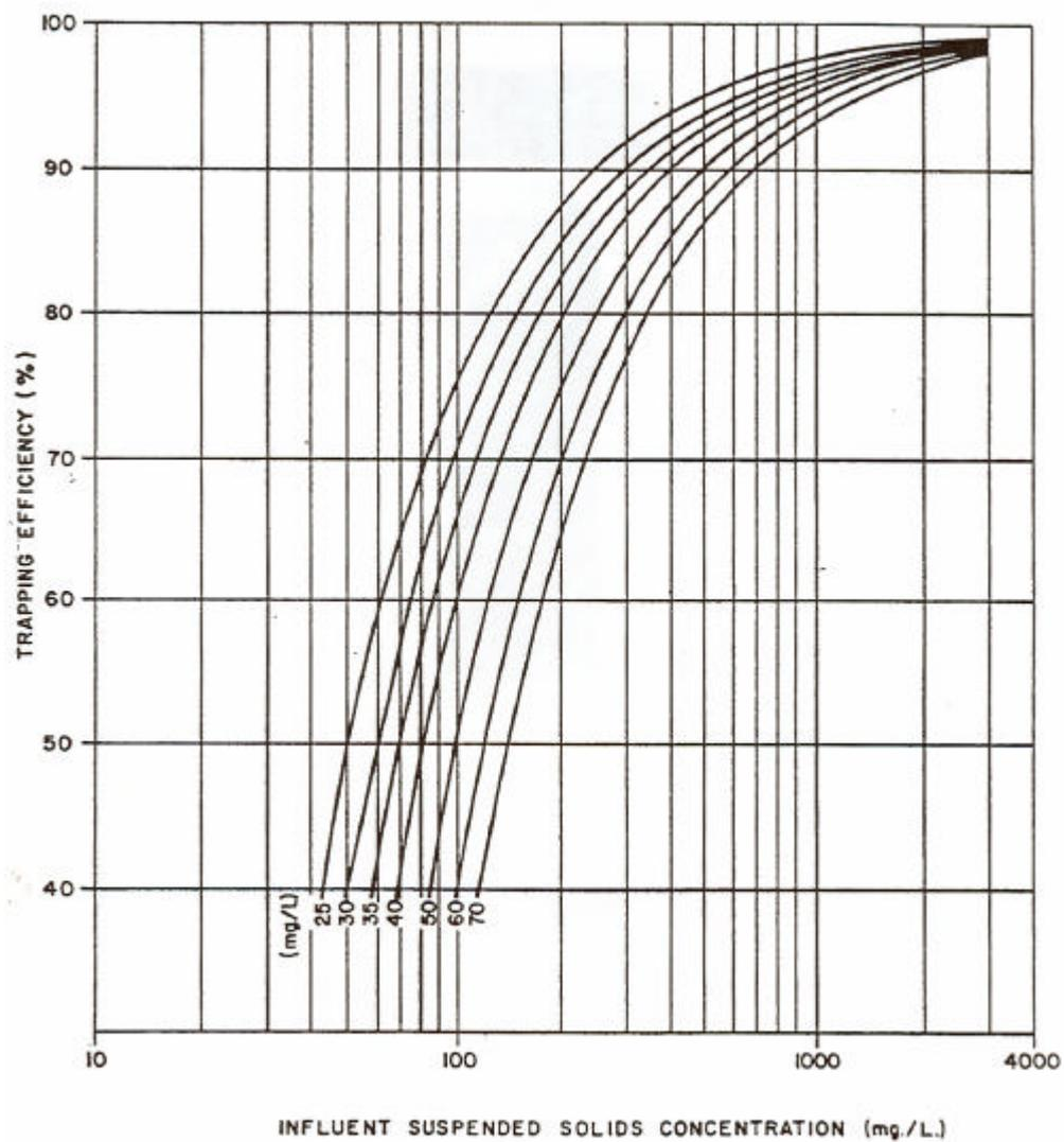
**Figure 4:1** Required trapping efficiency to Meet Various Effluent Limitations
