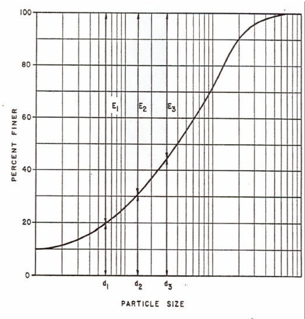
Figure 4:2 Definition of trapping Efficiency for Various Particle Sizes
