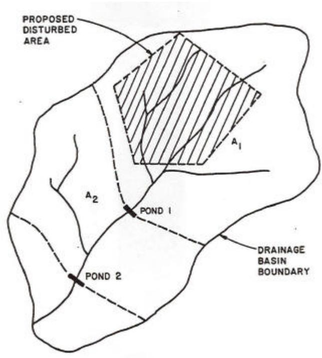
Figure 2.1 Schematic design for ponds in series
