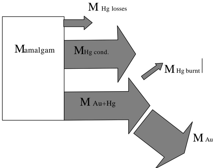
$$M_{\text{amalg.}} = M_{\text{Au+Hg}} + M_{\text{Hg cond.}} + M_{\text{Hg losses}} \quad (1)$$
