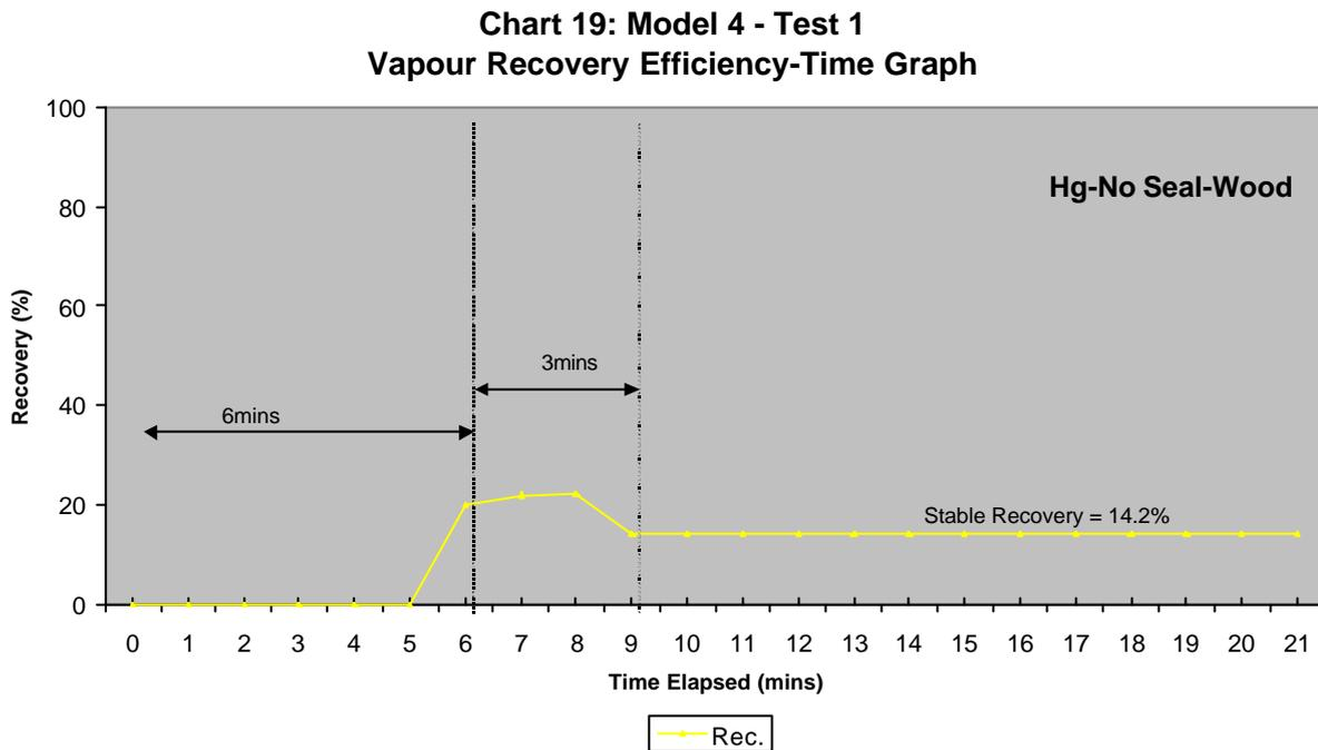
An open flame, created by burning a specie of hard wood in a fire containment structure, was used as the source of heat for this test. **Chart 19** shows that mercury condensate appeared approximately 6 minutes after commencement of the test and a stable condensate mass was attained approximately 3 minutes thereafter. Stable recovery was achieved 9 minutes after commencement of the test.
