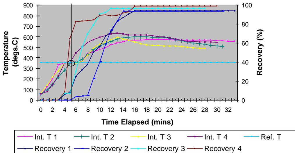
The achieved performance of this retort was obtained at average sustained internal and external temperatures 538.6 °C and 685.4 °C.
