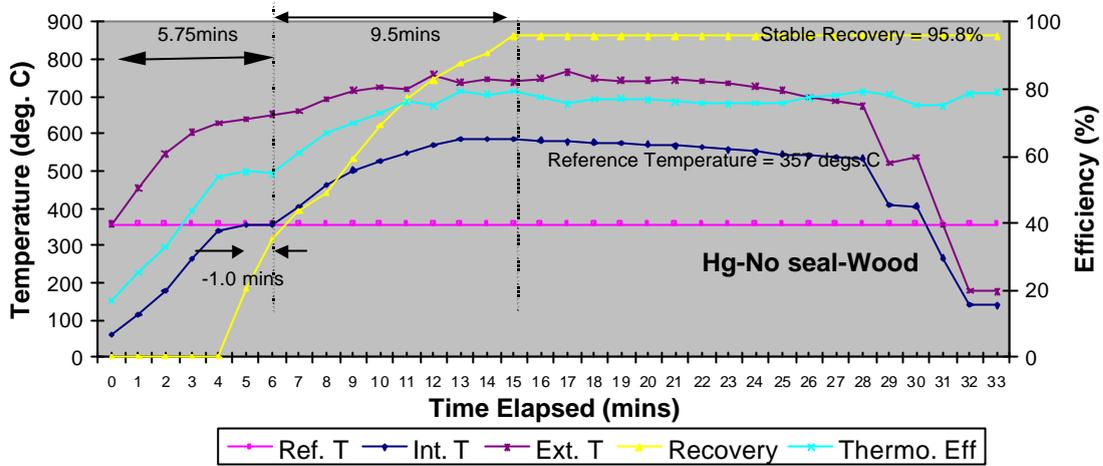
A comparison of the recovery and internal temperature shows a direct relationship between the two parameters i.e. mass accumulation mirrors closely the changes in internal temperature. This observation is clearly demonstrated in **Chart 9**. The clustered nature of the parameter graphs shown in **Chart 9** reflects the consistency in the retort performance, test procedures and to some extent the test conditions.
