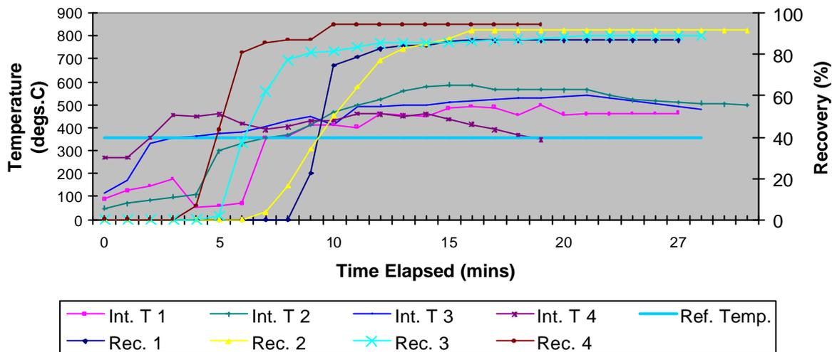
A comparison of the recovery and internal temperature shows a direct relationship between the two parameters i.e. mass accumulation mirrors closely the changes in internal temperature. This observation is clearly demonstrated in **Chart 5**. The clustered nature of the parameter graphs shown in **Chart 5** reflects the consistency in the retort performance, test procedures and to some extent the test conditions.
