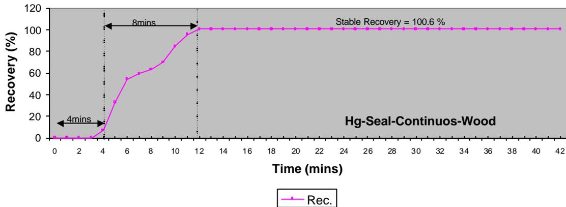
An open flame, created by burning a specie of hard wood in a fire containment structure, was used as the source of heat for this test. **Chart 13** shows that mercury condensate appeared approximately  $4.0 \pm 1.0$  minutes after commencement of the test and a stable condensate mass was attained approximately  $8.0 \pm 1.73$  minutes thereafter. Stable recovery was achieved  $12 \pm 2.65$  minutes after commencement of the test.
