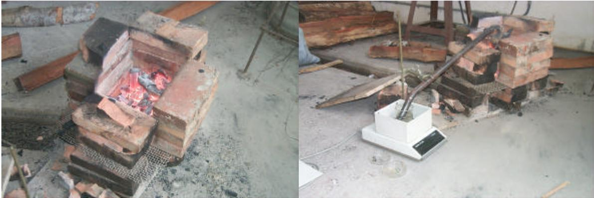
**Picture 7:** Charcoal in containment structure and retort placement for testing.
