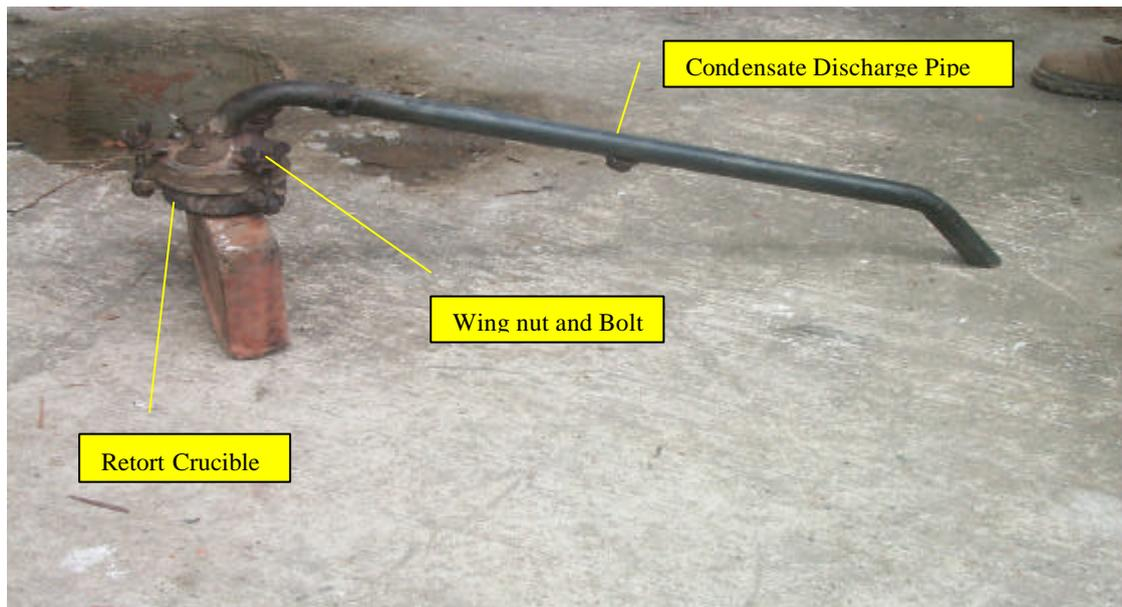
**Picture 5:** ED Model 3 Retort (GG&MC/GENCAPD Retort).
