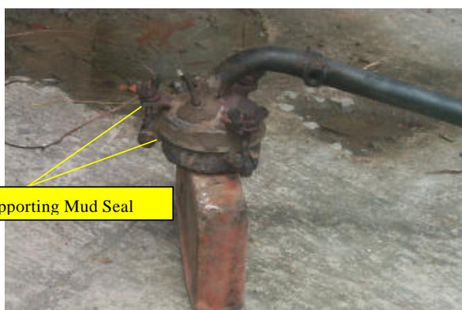
**Picture 3:** GG&MC/GENCAPD Retort showing placement of mud seal.
