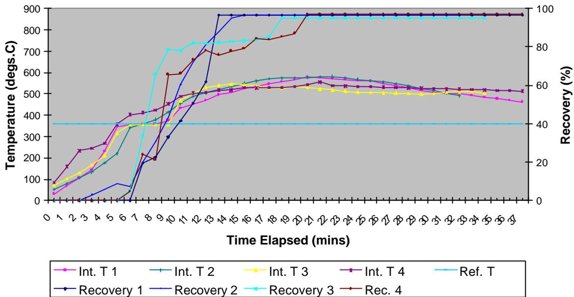
**Chart 11** also shows that the retort is most thermodynamically efficient when the internal temperature is above approximately 550 °C (external temperature above approximately 700 °C). Recovery peaks (optimum recovery) under these thermodynamic conditions.
