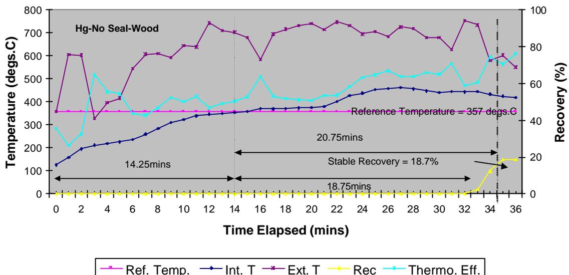
The achieved performance of this retort was obtained at average sustained internal and external temperatures 417.9<sup>0</sup>C and 636.4<sup>0</sup>C.
