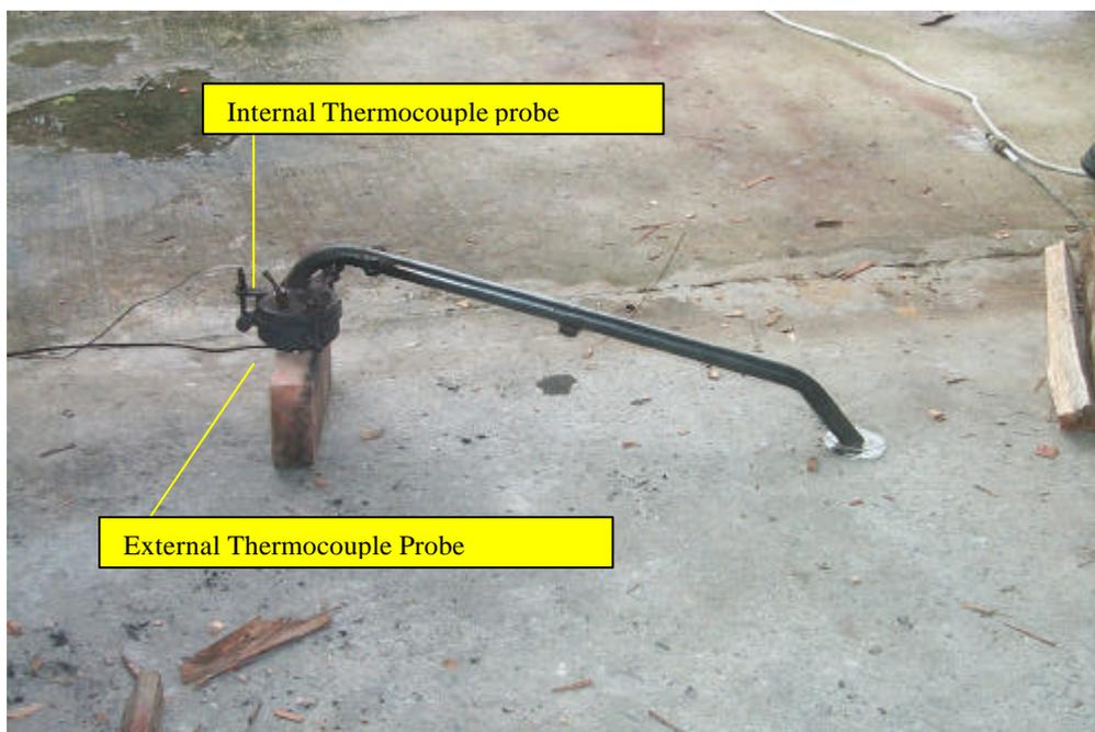
**Picture 1:** Placement of thermocouple probes with respect to the crucible
