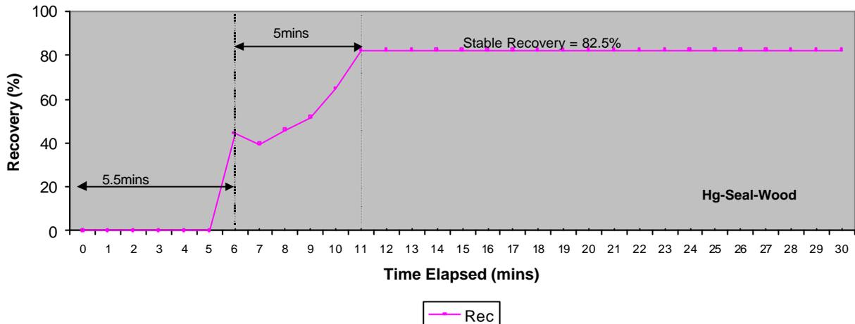
An open flame, created by burning a specie of hard wood in a fire containment structure, was used as the source of heat for this test. **Chart 20** shows that mercury condensate appeared approximately 5.5 minutes after commencement of the test and a stable condensate mass was attained approximately 5 minutes thereafter. Stable recovery was achieved 10.5 minutes after commencement of the test.
