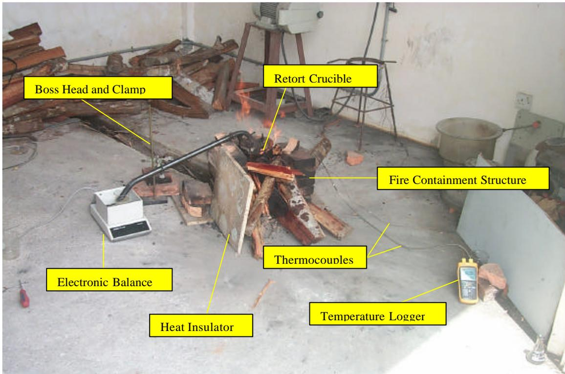
**Picture 4:** Showing testing in progress and placement of retort relative to fire containment structure and condensate collection unit
