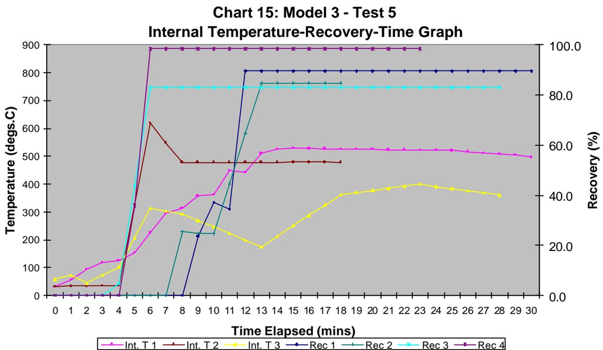
The achieved performance of this retort was obtained at average sustained internal and external temperatures  $456.8^{\circ}\text{C}$  and  $575.5^{\circ}\text{C}$ .
