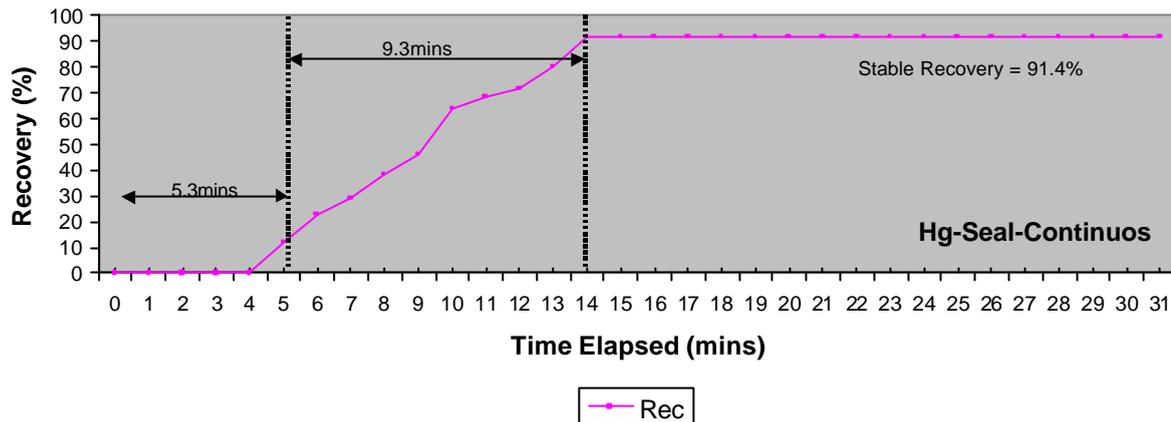
An open flame, created by burning a specie of hard wood in a fire containment structure, was used as the source of heat for this test. **Chart 6** shows that mercury condensate appeared approximately  $5.3 \pm 1.53$  minutes after commencement of the test and a stable condensate mass was attained approximately  $9.3 \pm 3.5$  minutes thereafter. Stable recovery was achieved  $14.7 \pm 5.03$  minutes after commencement of the test.
