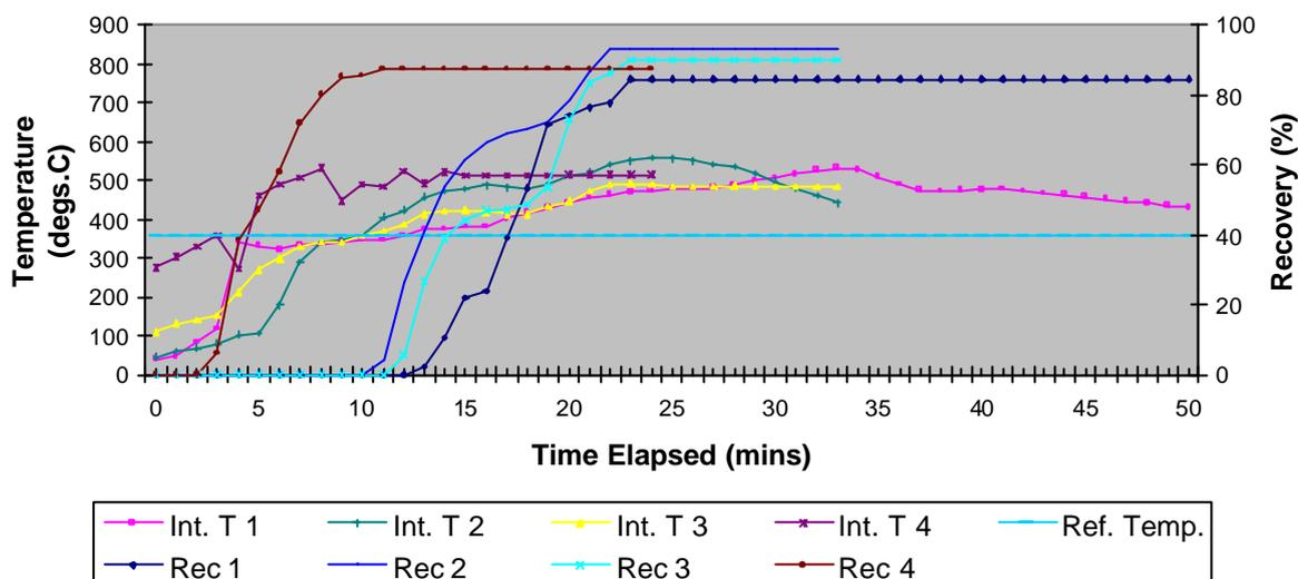
A comparison of the recovery and internal temperature shows a direct relationship between the two parameters i.e. mass accumulation mirrors closely the changes in internal temperature. This observation is clearly demonstrated in **Chart 3**. The clustered nature of the parameter graphs shown in **Chart 3** reflects the consistency in the retort performance, test procedures and to some extent the test conditions.
