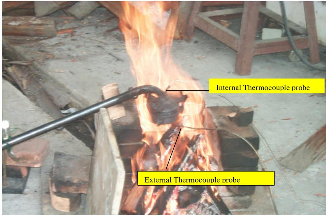
**Picture 2:** Placement of thermocouple probes with respect to the heat source.
