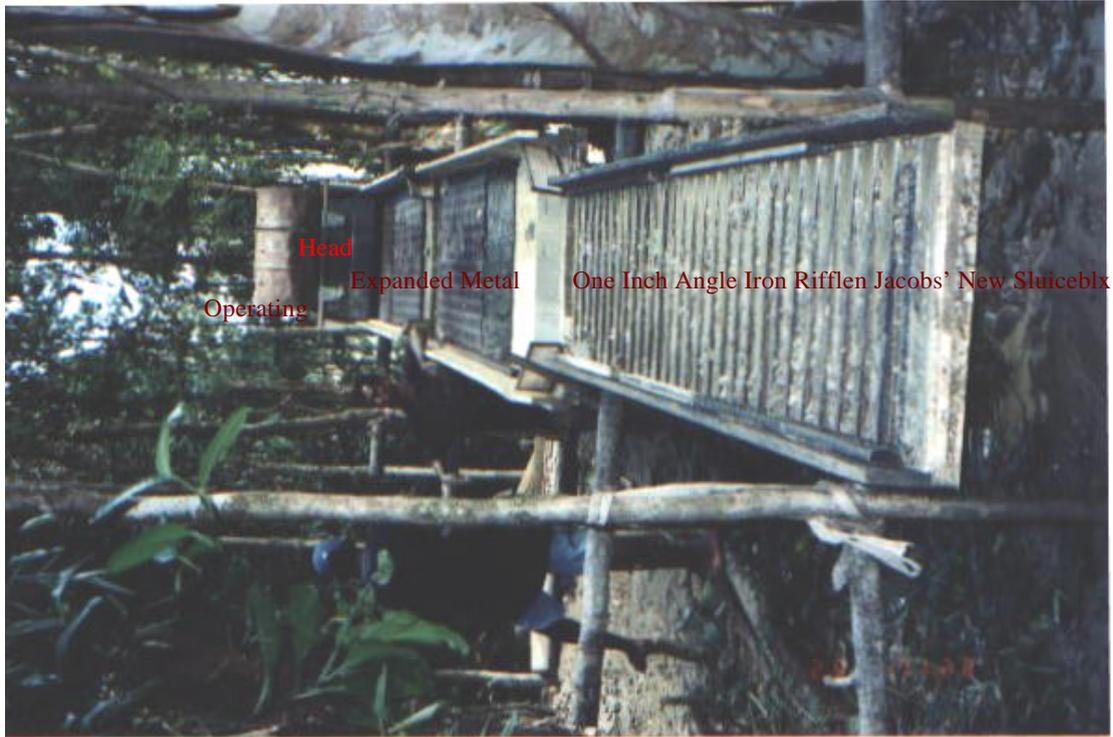
Photo 8 Collin Jacobs' New Sluicebox Operating
