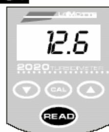
**7.** The 2020 will turn off automatically 2 minutes after the last button push. To turn the meter OFF manually, hold the **READ** button down for at least 1 second. Release the button when OFF is displayed.
