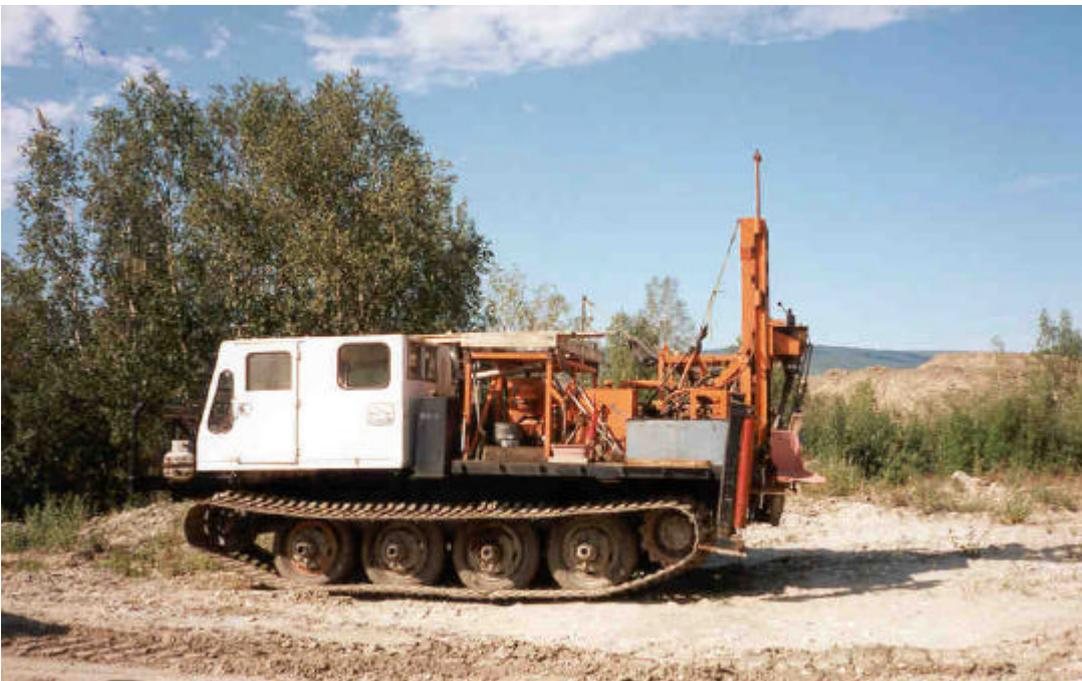
*GIMLEX Gold Mines: Nodwell All Terrain Low Ground Pressure Vehicle with Large Auger Drill*
