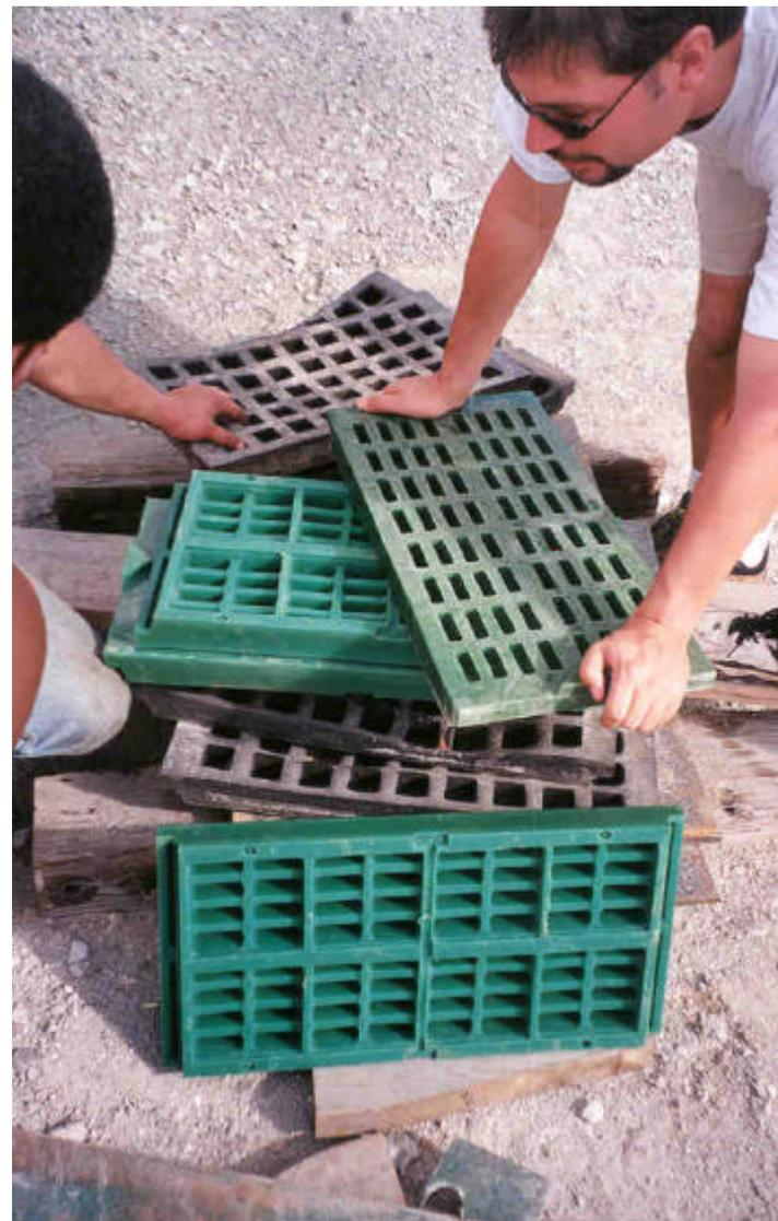
*Polyurethane Screen used for Vibrating Screen Deck (10-20 times longer wear resistance than woven wire mesh usually used)*
