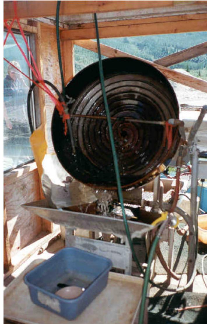
*GIMLEX Gold Mines, Large Custom-Built Rotary Gold Wheel for Final Cleaning*
