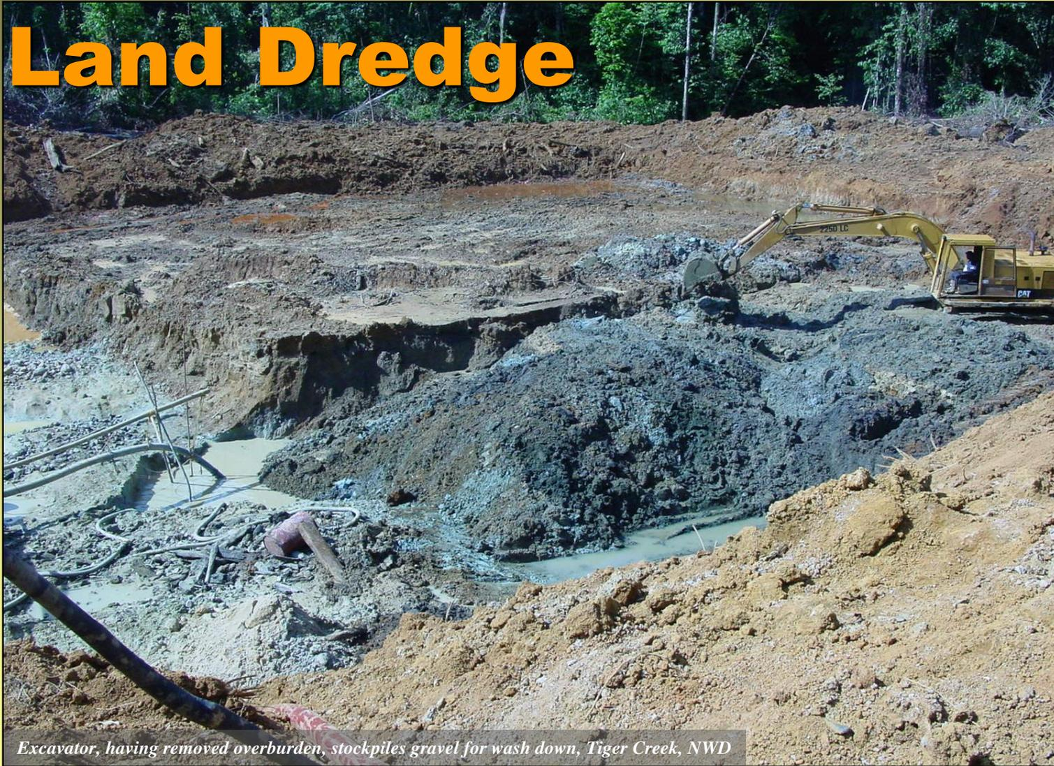
*Excavator, having removed overburden, stockpiles gravel for wash down, Tiger Creek, NWD*
