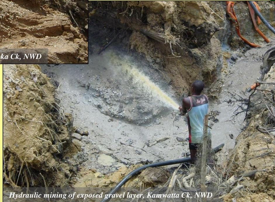
*Hydraulic mining of exposed gravel layer, Kamwatta Ck, NWD*
