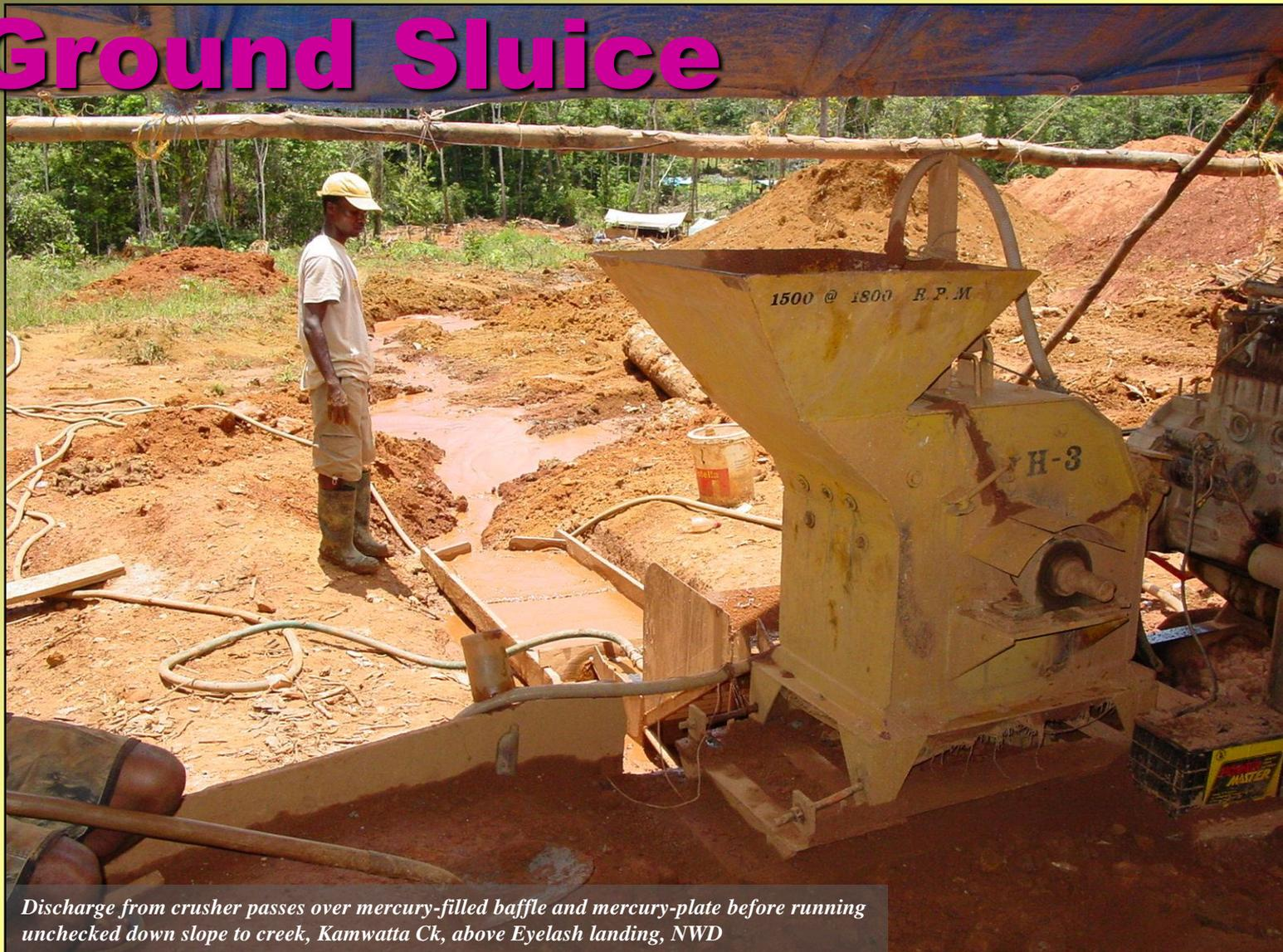
*Discharge from crusher passes over mercury-filled baffle and mercury-plate before running unchecked down slope to creek, Kamwatta Ck, above Eyelash landing, NWD*
