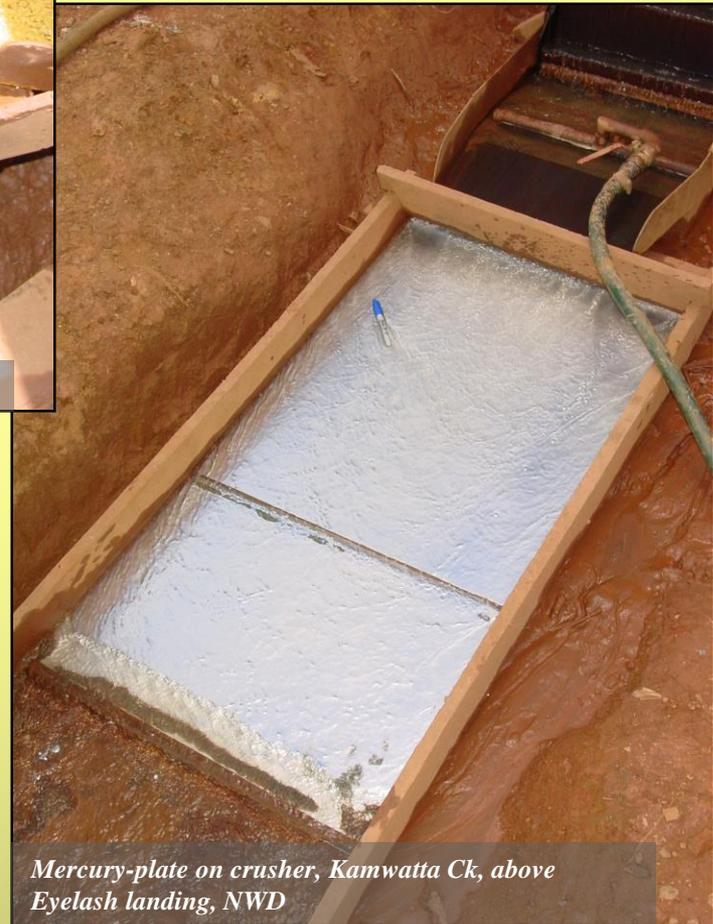
*Mercury-plate on crusher, Kamwatta Ck, above Eyelash landing, NWD*
