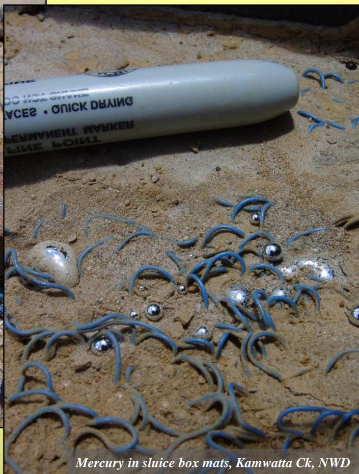
*Mercury in sluice box mats, Kamwatta Ck, NWD*
