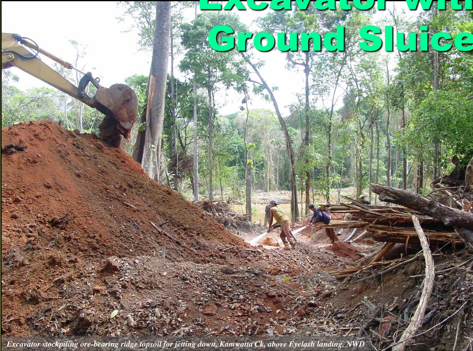
*Excavator stockpiling ore-bearing ridge topsoil for jetting down, Kamwatta Ck, above Eyelash landing, NWD*
