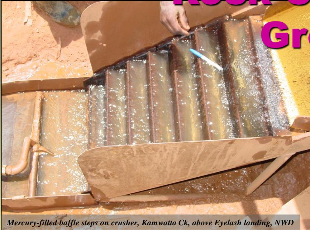
*Mercury-filled baffle steps on crusher, Kamwatta Ck, above Eyelash landing, NWD*
