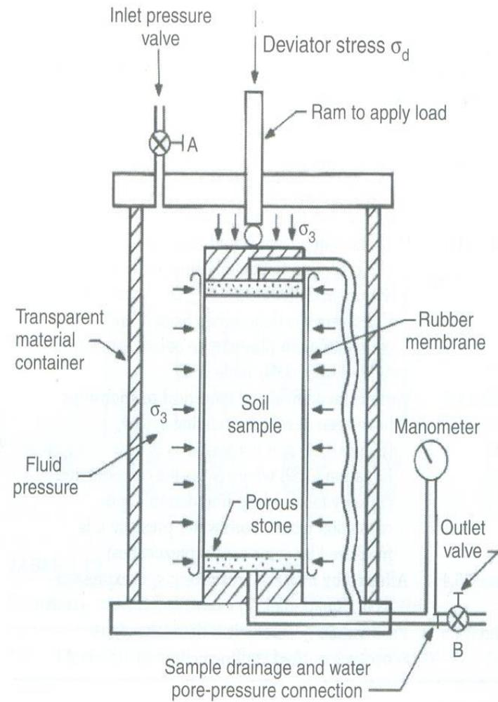
TRIAXIAL COMPRESSION APPARATUS AND CHAMBER ARRANGEMENT.
